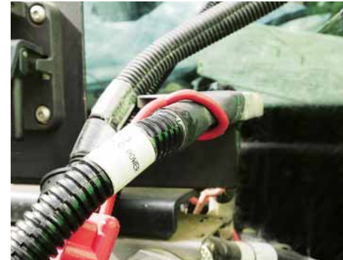
Connect the Power harness.
