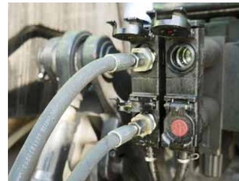
Connect the hydraulic hitch jack hoses to the tractor - labelled 'JACK UP' & 'JACK DOWN'.
