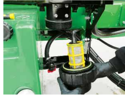
Unscrew the bowl nut, then carefully remove the filter screen & clean the filter bowl, body, screen & O-rings.
