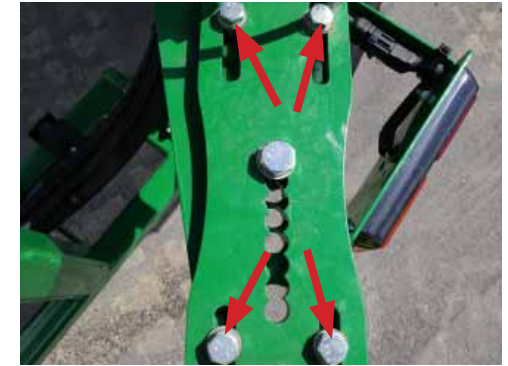
Loosen 4 corner bolts of the Cable Adjuster Plate.
