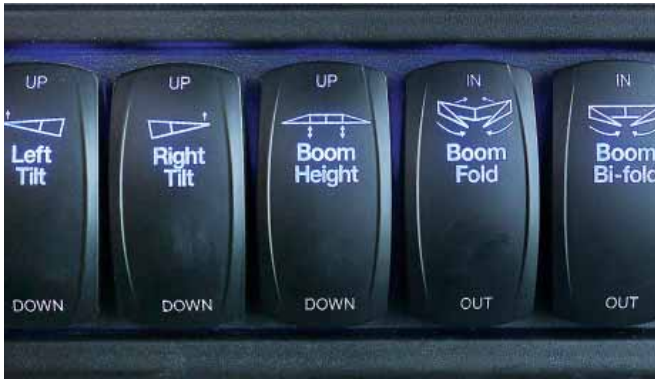
Switches on the Sprayer Switch Console are used to operate boom folding and unfolding functions.
