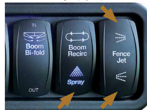
Press the 'Spray' push button to clean boom nozzles, as well as the left & right 'Spray Jet' push buttons.
