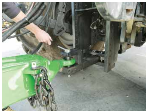
Reverse the tractor to align the tongue and drawbar holes, then fit the drawbar pin.
