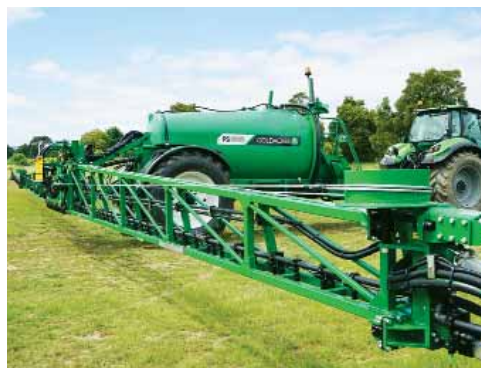
On level ground, engage tractor park brake, chock wheels & have the boom in working position before making adjustments.
