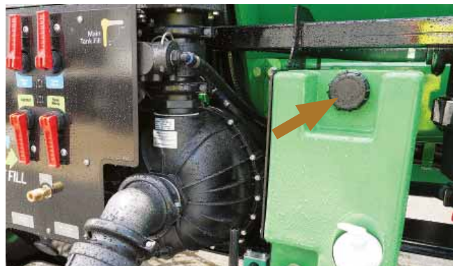
Remove the Hand Wash Tank fill cap to fill the tank with clean water only. Replace the cap when the tank is filled.
