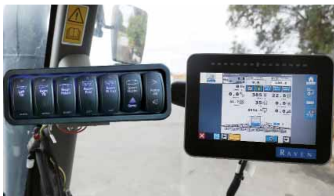
Standard In-Cab Sprayer Control Console (shown left) with Optional Raven Controller CR7 (shown right).
