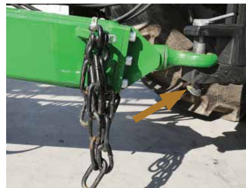
Ensure the drawbar pin is locked in position.
