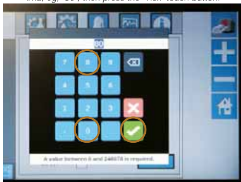
Press the appropriate touch buttons to set the 'Rate #1' in l/min, eg, '80', then press the 'Tick' touch button.
