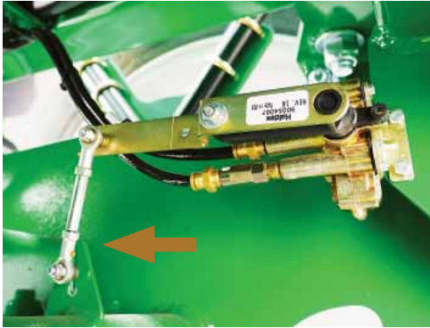
Adjustment to ride height is made by adjusting the linkage bolt in the slot where it attaches to the chassis.
