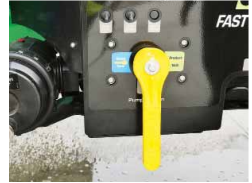
Before cleaning filters, rotate the 'Pump Suction' valve to Off position to isolate the Product Tank.
