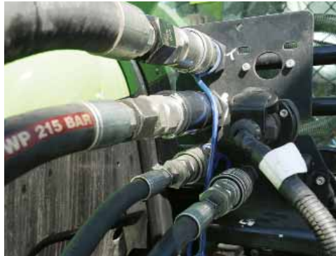
Connect the Tank, Pressure, Case Drain & Load Sensing hydraulic hoses to the tractor.
