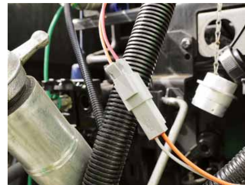
Connect the Master Switch connector.
