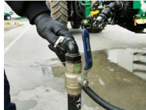
Open the Probe Valve to transfer chemical to the Hopper.
