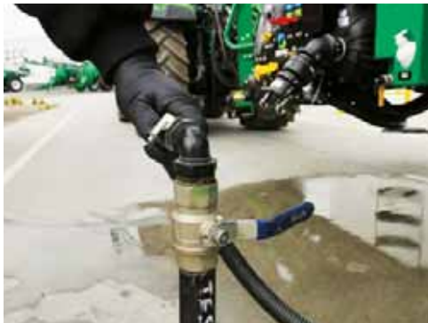
After completion of rinsing close the Probe Valve.
