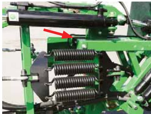
Rear view of Tilt Arm Guide wear pads - RHS boom.
