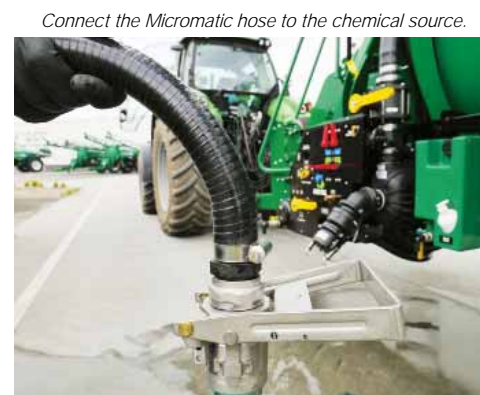
Connect the Micromatic hose to the chemical source.
