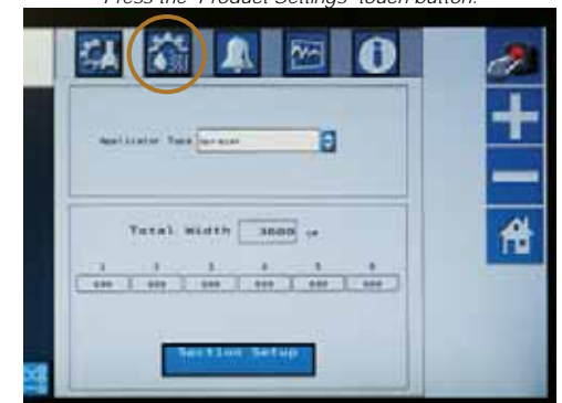
Total Width & Section Widths are displayed. Press the 'Product Settings' touch button.
