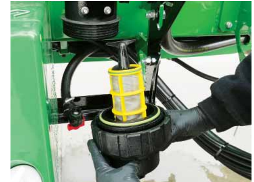
Carefully remove the Pressure Filter screen for washing & cleaning.
