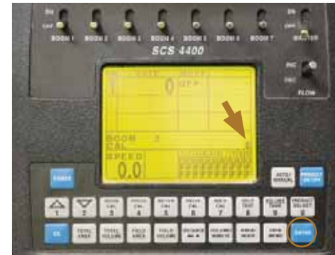
BOOM CAL 2: Press the 'ENTER' touch button to display the 'E' symbol in the lower RHS of the calibration screen.
