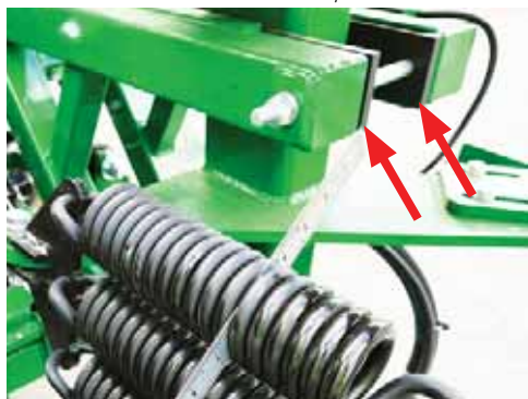
Front view of Tilt Arm Guide wear pads - RHS boom.
