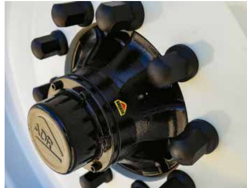
Recommended wheel nut torque tension is 320 ft/lb.
