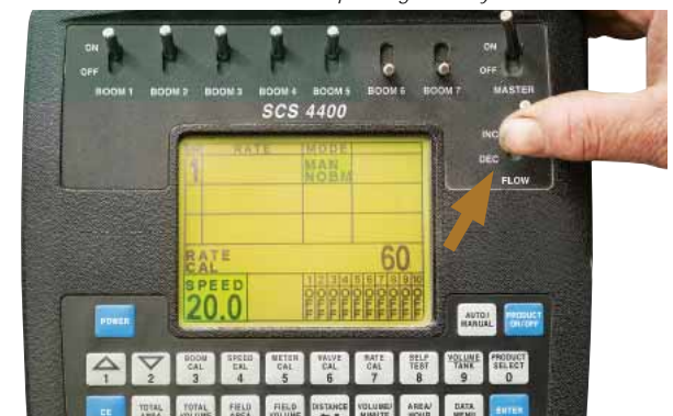
Use the 'FLOW' toggle switch to 'INC' then 'DEC' spray application rate to check the flow control valve is operating correctly.
