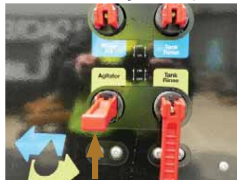
Check the main tank 'Agitator' valve is open.
