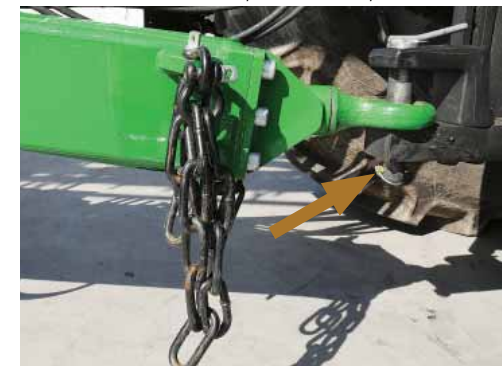
Ensure the drawbar pin is locked in position.
