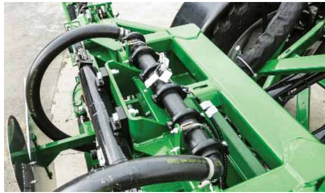
The Flow Meter, located on top of the boom centre section, should regularly inspected & cleaned.
