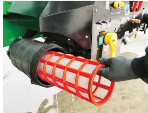
Carefully remove the filter screen, then clean the filter bowl, body, screen & O-rings.
