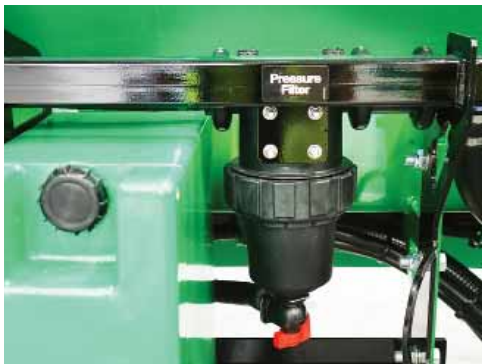
The Pressure filter located at the Fast Fill Station.
