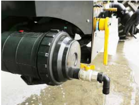
Open the drain valve of the Suction Filter.
