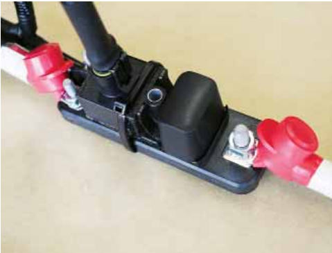
The main power fuse of the Prairie Special electrical system is fitted near the tractor battery.
