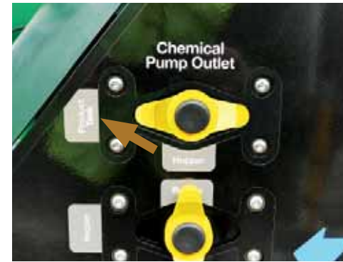
Rotate the 'Chemical Pump Outlet' valve to 'Product Tank'.
