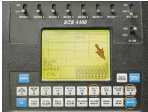
BOOM CAL 1: Press the 'ENTER' touch button to display the 'E' in the lower RHS of the calibration screen.
