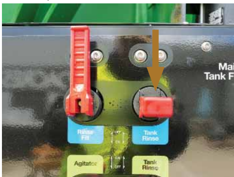
Open the fresh water 'Tank Rinse' valve.
