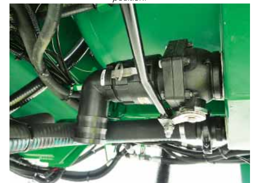
Main Tank Drain Valve (underneath the sprayer) in closed position.
