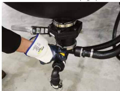
Close the Bottom Drain Valve, disconnect the micromatic hose & refit the camlock coupling cap.
