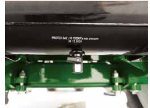
Air tank drain valve.
