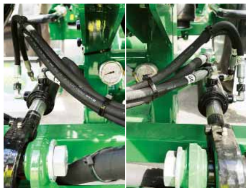
Two Yaw hydraulic cylinders (located on the boom centre section) & an accumulator form the independent pressurised Yaw hydraulic circuit.
