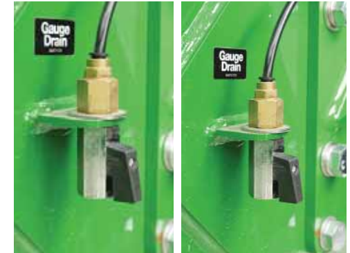
Gauge Drain valve closed (shown left) & Gauge Drain valve closed (shown right).
