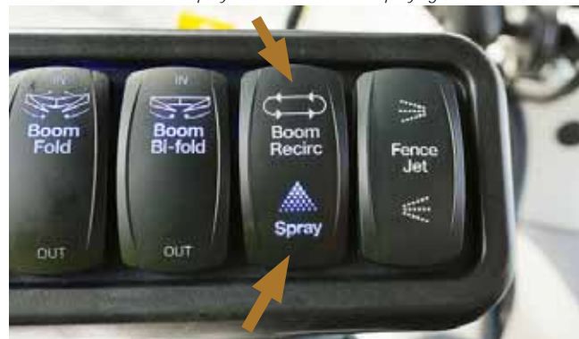
Start the 'Product Pump', then press the 'Boom Recirc' switch 'On', then switch to 'Spray' to start the nozzles spraying.
