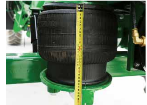
Left hand airbag inflated is 250mm (10"). Measure from the base of the top plate to the bottom of the airbag.
