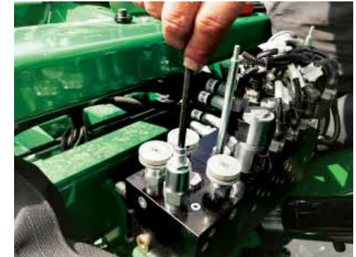
Set the Yaw Pressure with the Pressure Reducing Valve, then re-tighten the locknut.
