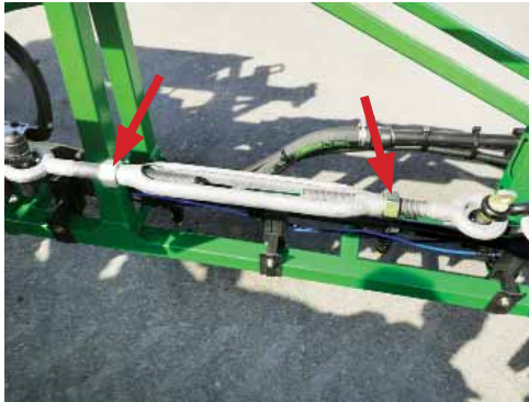
Undo the locknuts of the Cable Eyebolt Adjuster, then rotate the adjuster to tension the cable & retighten the locknuts.
