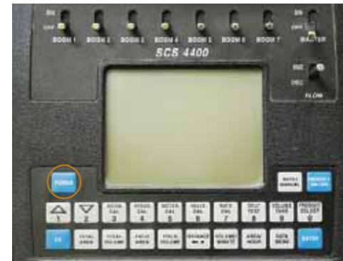
Press the 'POWER' touch button to start the Controller.
