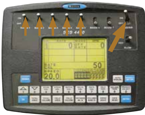
Boom section On/Off Toggle Switches & Boom Master On/Off Toggle Switch on the optional SCS 4400 Controller.
