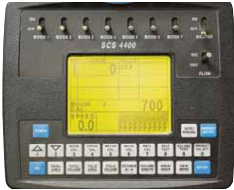
Check Boom Width & Boom Section Width values saved in the optional SCS 4400 Controller.
