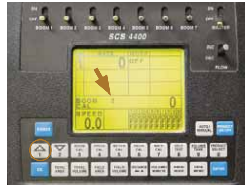
Press the 'UP' touch button to display the 'BOOM CAL 2' for Section 2 calibration.
