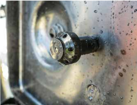
The Hopper Rinse Nozzle located under the hopper lid.
