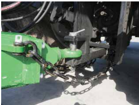
Connect the safety chains to the tractor & fully tighten the D-Shackle bolts.
