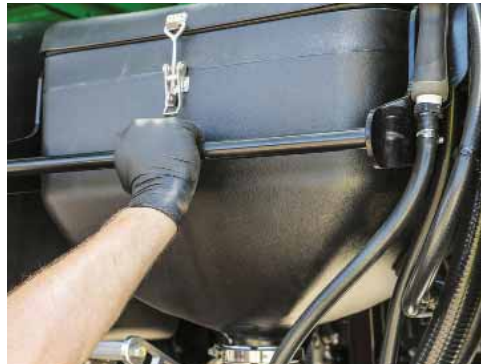
Support the hopper weight while unlocking the latch lever, then lower the hopper to its working position.
