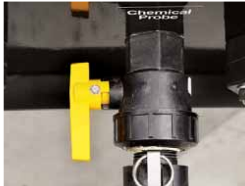
Open the Chemical Probe inlet valve.
