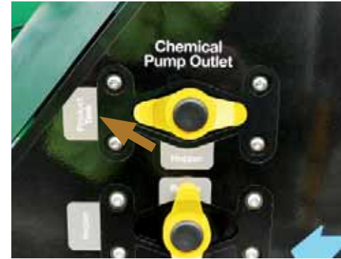
Rotate the 'Chemical Pump Outlet' valve to 'Product Tank'.
