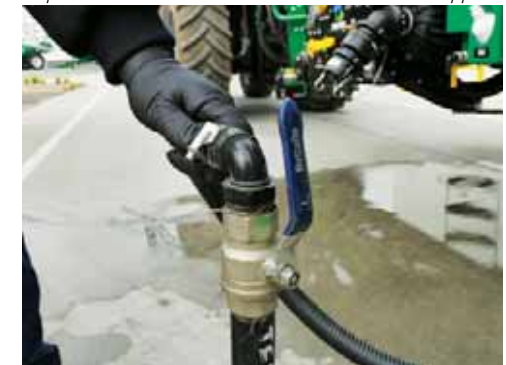
Open the Probe Valve to transfer chemical to the Hopper.
