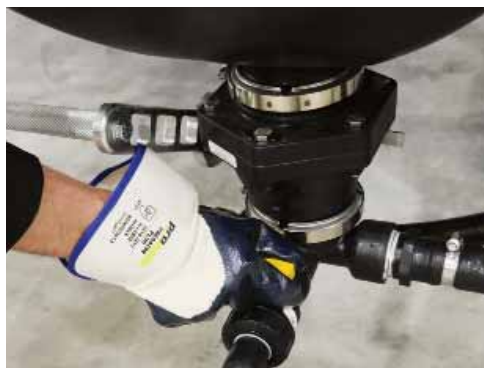
Open the Bottom Drain Valve to transfer chemical to the main tank.
