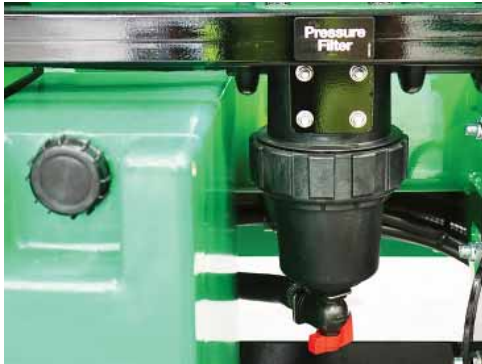
Fresh water tank (left) & Pressure Filter (right).
