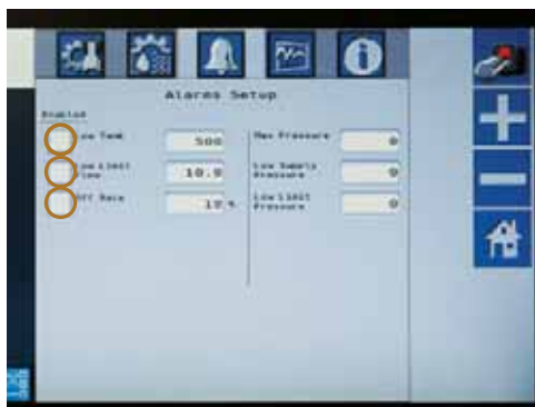
Press desired alarm touch buttons to enable or disable alarms.
