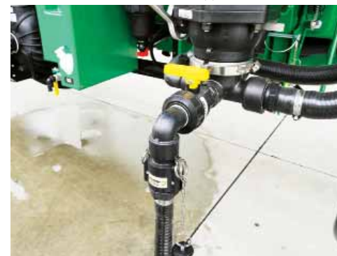
Push-Down to Close the foot operated ball valve at the base of the hopper.
