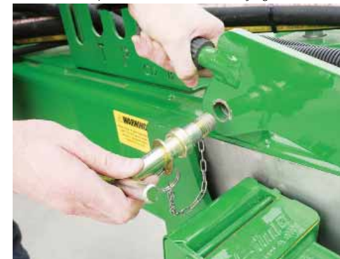
Rotate the hitch jack to the transport position, then replace the lock pin & screw-in until it is fully tightened.
