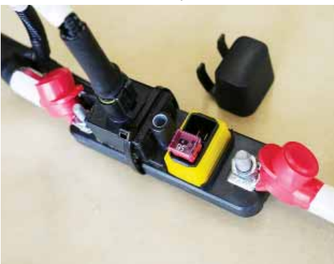
The main fuse of the electrical system with cover removed.
