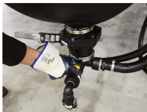
Close the Bottom Drain Valve, disconnect the Chemical Probe hose & refit the camlock coupling cap.
