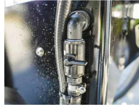
Access the Drum Rinse Nozzle.
