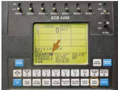
Press the 'DATA MENU' touch button to display the Data Sub Menus - 1st displayed & highlighted is 'SERIAL'.
