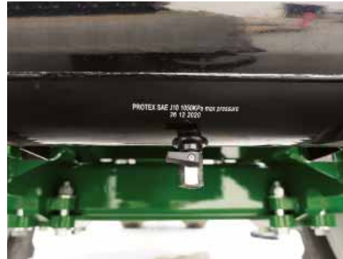
Manual drain valve (at the base of the Air Tank) in closed position.
