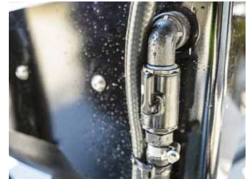
Open the Mixing Jet valve on the RHS of the Hopper.
