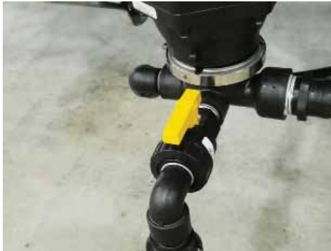
Open the Bottom Drain Valve for transferring chemical to the product tank.
