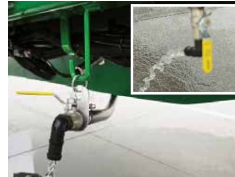
Unhook & open the Sump Drain Valve - lowering it to completely empty the main tank sump.
