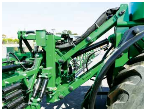
Goldacres Parallift Rear connection to the boom.
