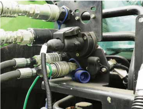
Connect the Tail Light harness.
