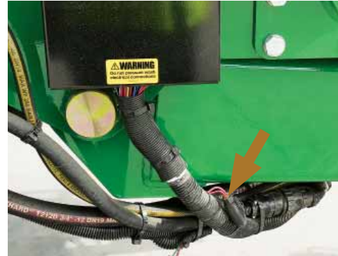
The RCM ISO BUS Control Centre fuse located on the harness.
