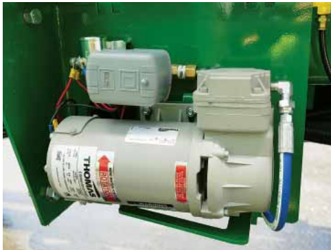
Air compressor located on the left hand side of the sprayer.
