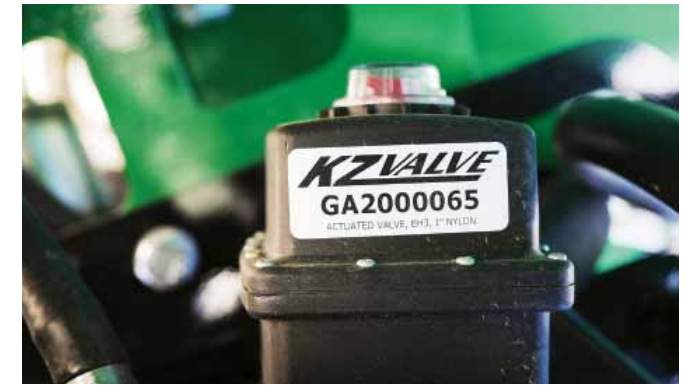
The Boom Flow Regulating Valve should regularly checked & calibrated.
