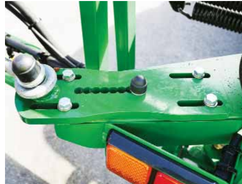
LHS Cable Adjustment Plate.
