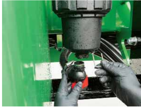
Remove the holding pin & disconnect the Red On/Off valve from the base of the pressure filter.
