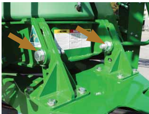
With the chassis and hitch firmly supported, loosen & remove the hitch angle adjustment bolts.
