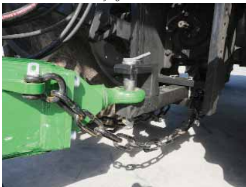
Unswcrew the safety chains D-shackles & connect them to the tractor, then fully tighten the D-Shackle bolts.
