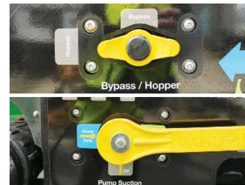
Rotate the 'Bypass/Hopper Valve' to Hopper and the 'Pump Suction Valve' to Product Tank position.
