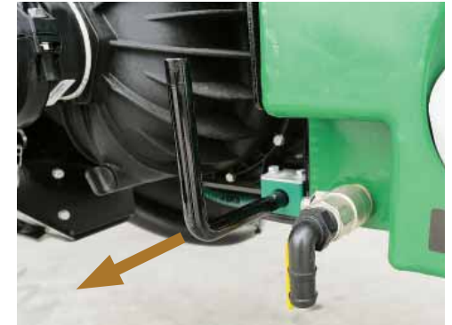
Pull out the 'Main Tank Drain Valve Lever' to safely & completely drain the Product Tank, then close the valve.
