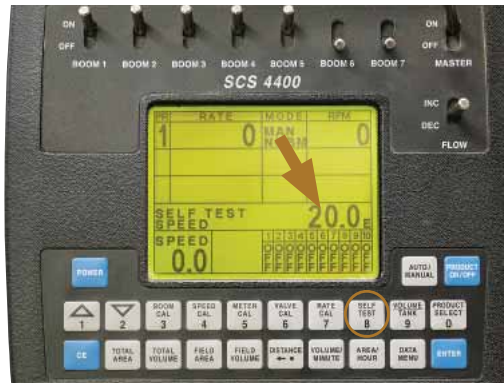
Press the 'SELF TEST' touch button, then enter & save normal operating speed, eg, 20km/hr.
