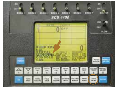
Press the 'DATA MENU' touch button to display the Data Sub Menus - 2nd displayed & highlighted is 'PRODUCT'.
