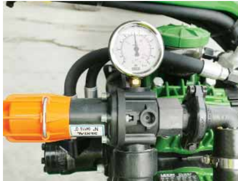
Pressure relief valve located on the diaphragm pump.
