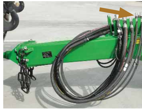
Reverse the tractor close enough to connect the hydraulic hitch jack hoses (shown by arrow above) to the tractor.
