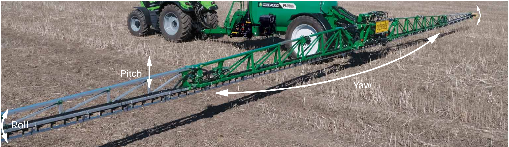
Goldacres' TriTech booms feature a unique three directional suspension system.
