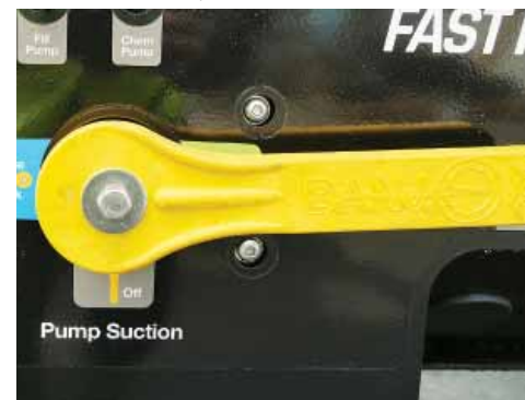
Return the 'Pump Suction Valve' to 'Product Tank'.
