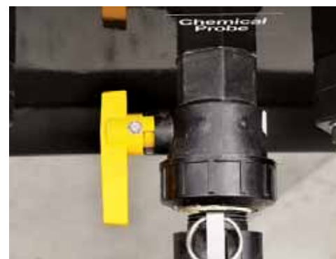
Connect the Micromatic hose & Open Chemical Probe inlet valve.
