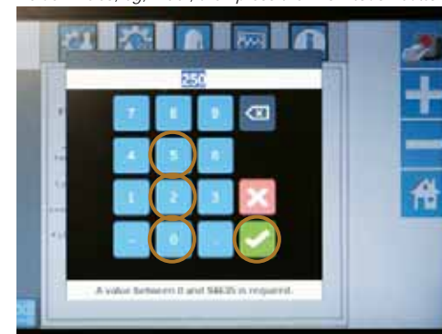
Press the appropriate touch buttons to set the 'Low Tank' value in litres, eg, '250', then press the 'Tick' touch button.
