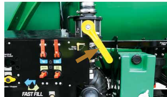
Partially close the 'Main Tank Fill Valve' to increase flow for other filling & cleaning functions.
