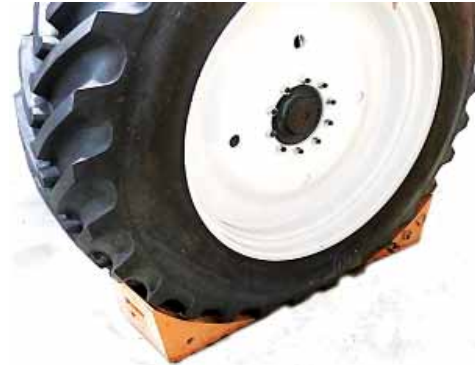
Chock opposite wheel of the sprayer before raising the other wheel off the ground.
