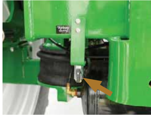
Open the Airbag Dump Valve to lower a sprayer for trailer transport & end of season storage.
