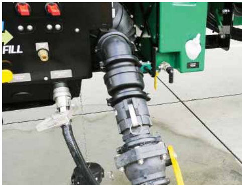
Connect the Micromatic hose coupling to the 'Micromatic Rinse' outlet on the Prairie Special.
