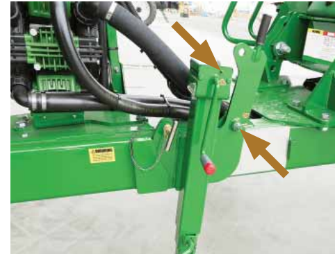
Grease the manual hitch jack.
