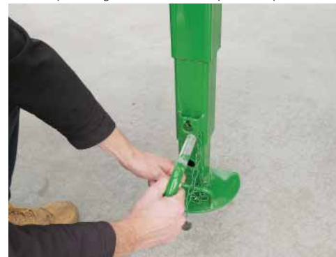
Raise the base plate by removing the pin, lift up the base plate, align the holes, then replace the pin.
