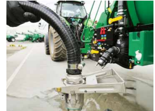
Connect the Micromatic hose to the chemical source.
