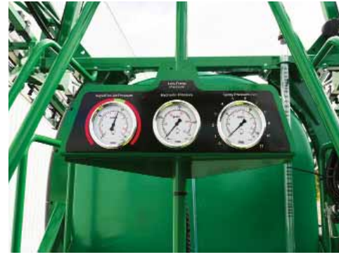
Check air, hydraulic & spray operating pressures.
