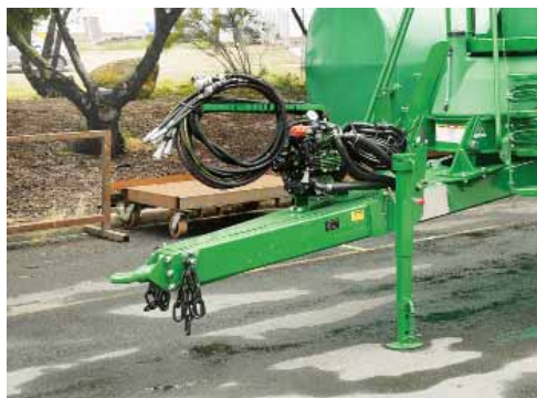
Hitch tongue & Manual Hitch Jack.
