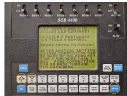
Adjust screen contrast, then press 'Enter' touch button to save the setting.
