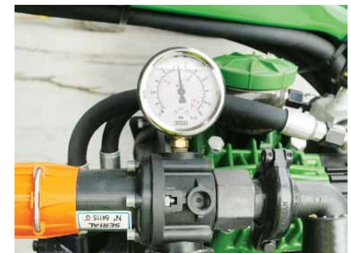
Operate pump speed to generate at least 80 psi (with hopper valves open).
