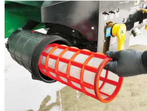
Carefully remove the Suction Filter screen for washing & cleaning.
