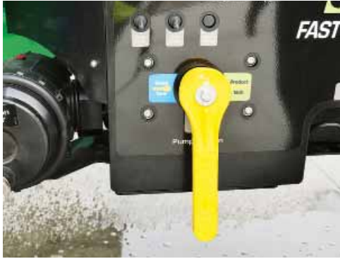
Before cleaning filters, rotate the 'Pump Suction' valve to Off position to isolate the Product Tank.
