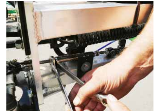
Check the lower pivot plates are properly aligned.
