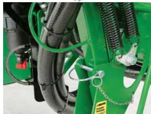
Raise the Hopper, then refit the locking pin & locking pin clip.
