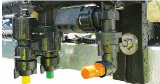
Selected & fit the appropriate nozzles for the application.
