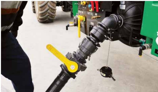
Connect a 3" suction hose to the 'Clean Fill Inlet'.
