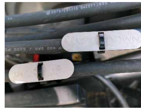
Locate the hydraulic hitch jack hoses to the tractor - labelled 'JACK UP' & 'JACK DOWN'.
