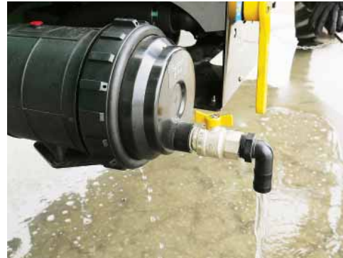
Open the drain valve to drain the Suction Filter.
