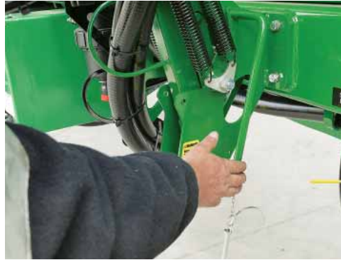
Remove safety pin & lifting arm locking pin. Support hopper weight, pull the latch lever to unlock, then lower the hopper.
