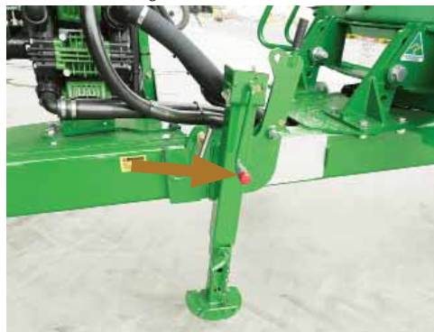
Rotate the hitch jack handle anti-clockwise to lower the hitch tongue onto the tractor drawbar.
