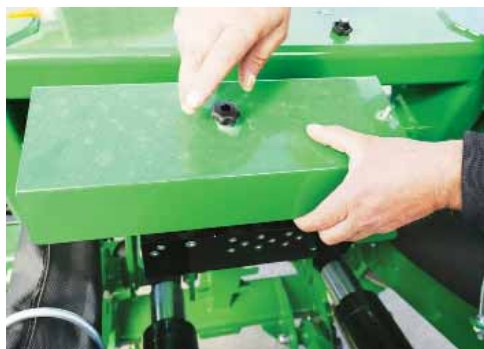
Remove the hydraulic manifold cover to access the adjustment valves.
