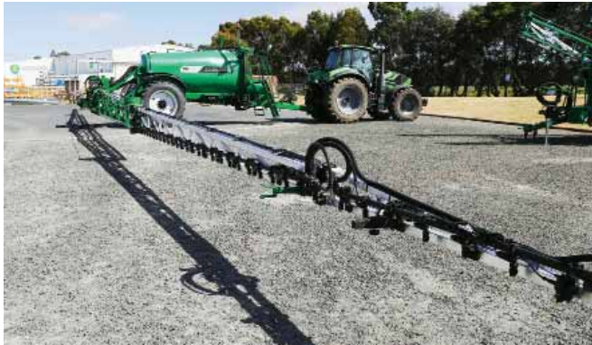
Unfold the boom in a suitable area & set the height of the boom to allow easy access to nozzles.
