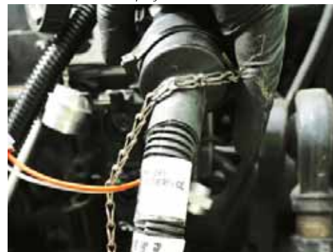
Connect Sprayer Console harness.
