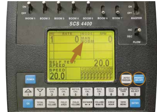
Press the 'SELF TEST' touch button, then enter & save normal operating speed, eg, 20km/hr.
