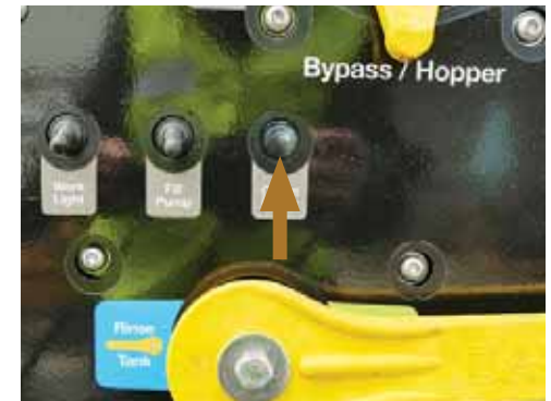
Switch Off the 'Chemical Pump'.
