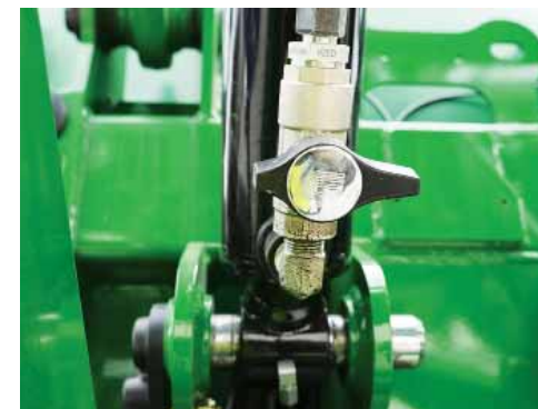
Close the ball valve on each lift cylinder (2) for safety.
