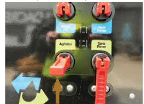
Open the main tank 'Agitator' valve.
