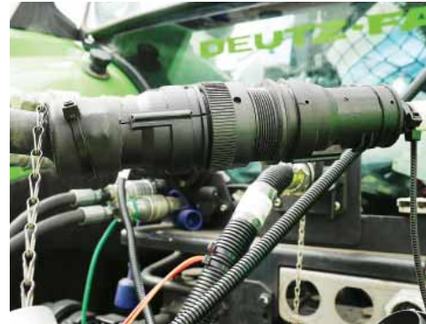
Connect the Control harness.
