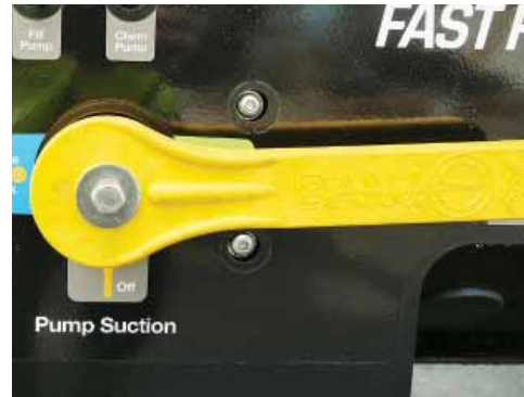
Rotate the 'Pump Suction Valve' to 'Product Tank'.
