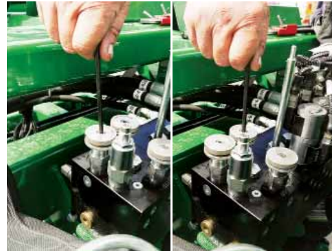
Loosen the locknuts, then wind out (counterclockwise) both 'Yaw A' & 'Yaw B' valves until fully open.
