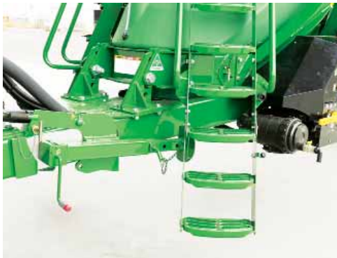
The hitch jack in transport position.
