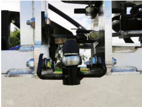
Check the lower pivot plates are properly aligned.
