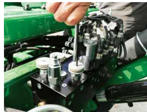
Loosen the locknut, then wind out (counterclockwise) the 'Yaw Bleed Valve' until fully open.
