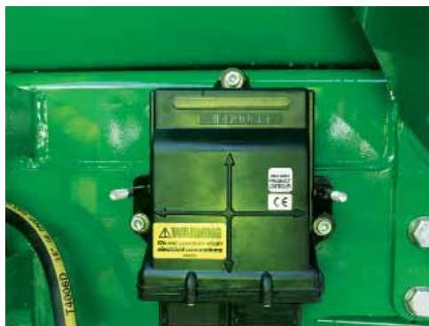
The Raven PC1 ISO BUS Control Centre, located on the LHS side on the sprayer chassis.
