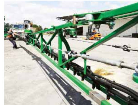
Use an assistant to pull back the outer boom arm to release tension on the cable.
