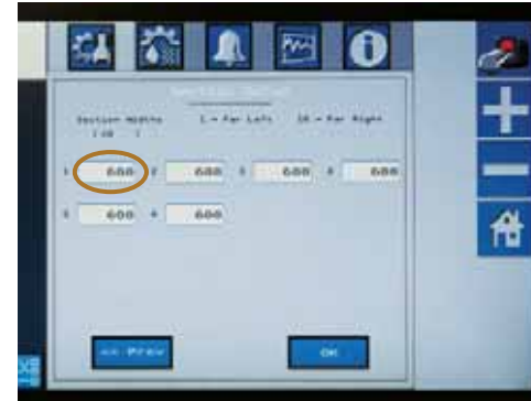
Press the 'Section 1' touch button to enter the width of Section 1.
