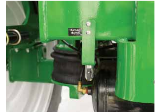
Deflate the air-bag suspension system for more load stability when loading & transporting the sprayer.
