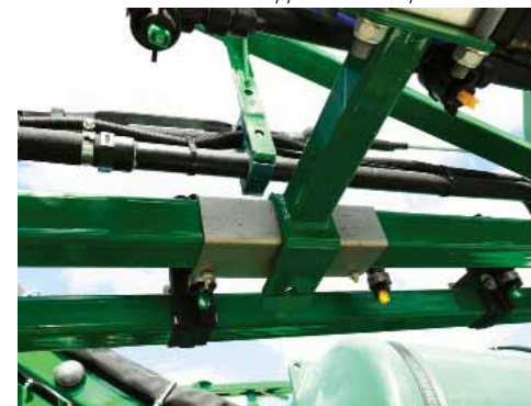
Outer boom saddle support in folded position.
