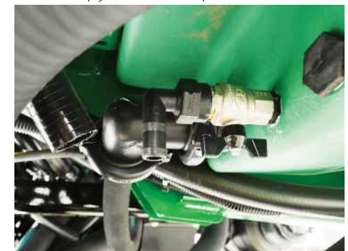
To empty the Rinse Tank, open its drain valve.
