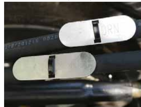
Each hydraulic hose is tagged for easy recognition - Case Drain & Load Sensing hose tags shown below.
