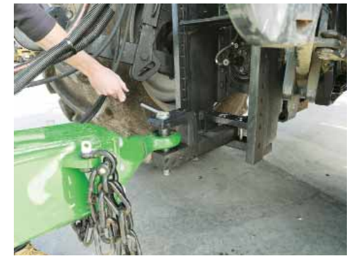
Reverse the tractor to align the tongue and drawbar holes, then fit the drawbar pin.
