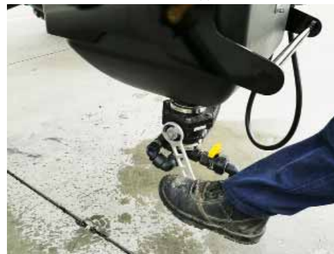
Push-Down to Close the foot operated ball valve at the base of the hopper.
