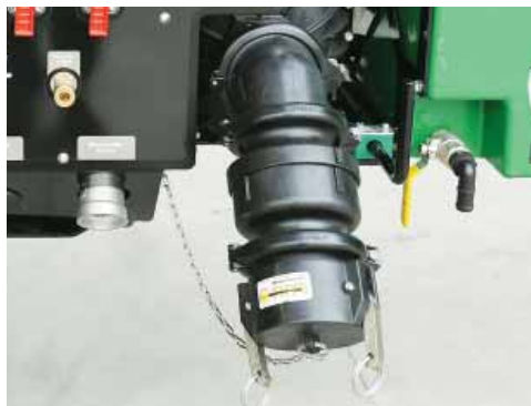
The 3" Clean Fill inlet camlock cap fitted.
