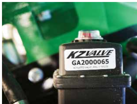
Flow Control Valve located under the Fast Fill station cover.
