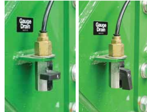
Gauge Drain valve closed (shown left) & Gauge Drain valve open (shown right).
