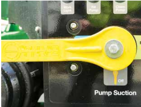
Rotate the 'Pump Suction Valve' to 'Rinse Tank'.
