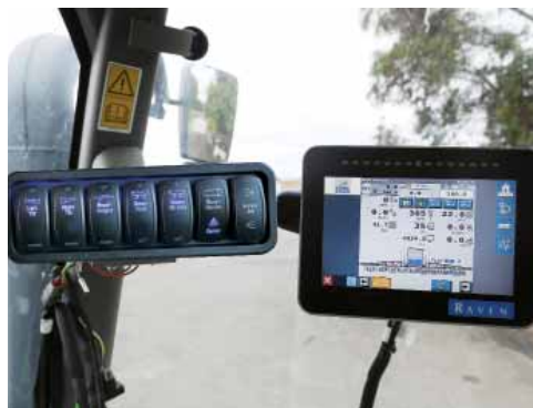
In-cab Sprayer Control Console (left) & optional Raven CR7 Controller (right).
