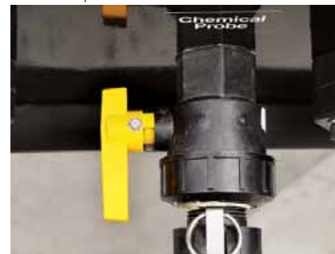
Open the Chemical Probe inlet valve.
