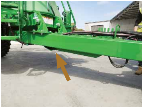
Fully raise the hitch jack & its base until it rests neatly under the sprayer hitch.
