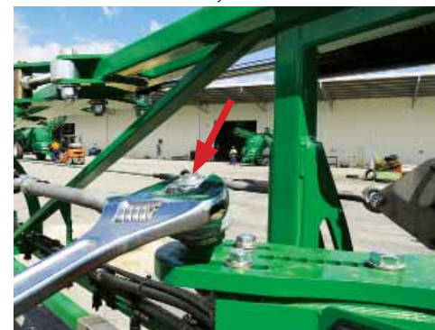
Undo the nut & remove the end of the Cable Turnbuckle Adjuster.
