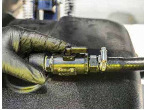
Open the Rinse Valve on top of the hopper lid.
