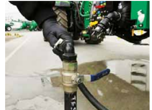
After completion of rinsing close the Probe Valve.
