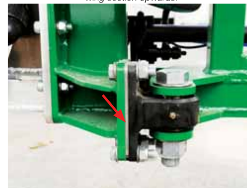
Add shims to the lower joint bracket to tilt the end of 2nd wing section upwards.
