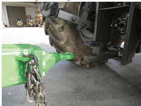
Manually wind the Hitch Jack up or down to match the hitch tongue to the height of the tractor drawbar.
