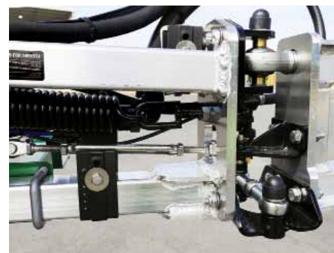
Three Way Tip Breakaway mechanism of the Trittech boom.
