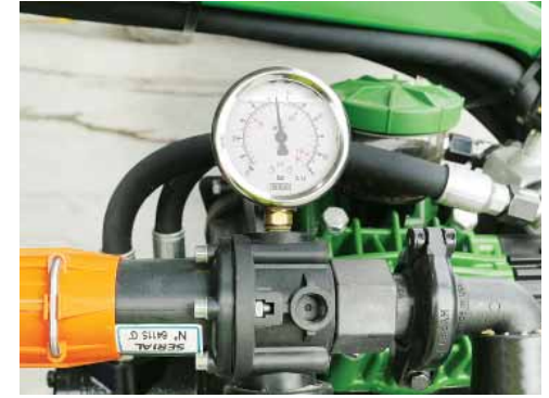
Operate pump speed to generate at least 80 psi (with hopper valves open).
