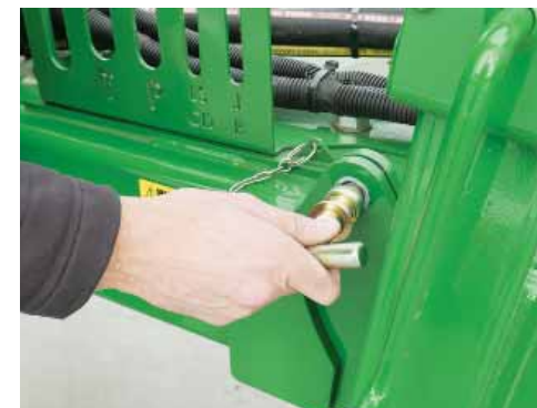
Unscrew & remove the hitch jack lock pin.
