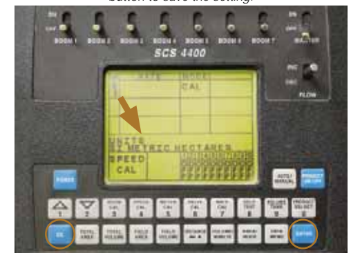
Scroll to 'SI METRIC HECTARES', then press 'Enter' touch button to save the setting.
