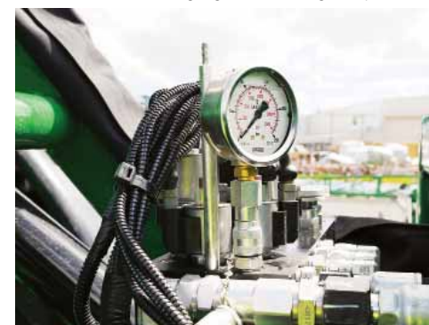
Use the Yaw Pressure gauge when setting Yaw pressure.
