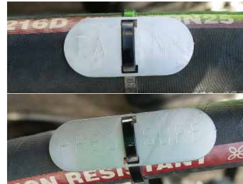
Each hydraulic hose is tagged for easy recognition - Tank & Pressure hose tags shown below.
