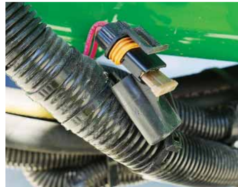
The ISO BUS Control Centre fuse with cover removed.
