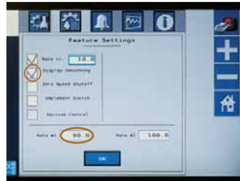
Press 'Display Smoothing' touch button to activate Display Smoothing. Press the 'Rate 1' touch button
