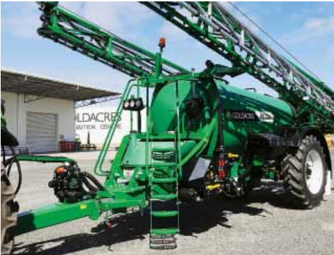
Empty the spray tank, park on a flat area, ensure the boom is closed and chock wheels before lifting a sprayer.
