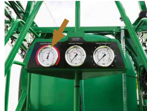
Air gauge showing RapidFire pressure on the left hand side at the front of the sprayer.
