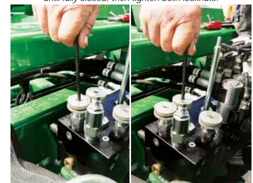
Close (wind-in [clockwise]) both 'Yaw A' & 'Yaw B' valves until fully closed, then tighten both locknuts.
