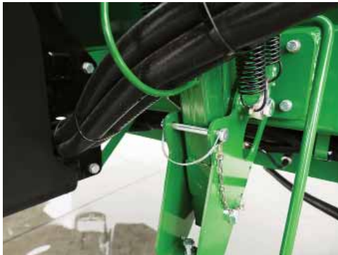
To lower the Chemical Induction Hopper, remove the hopper safety pin & locking pin.
