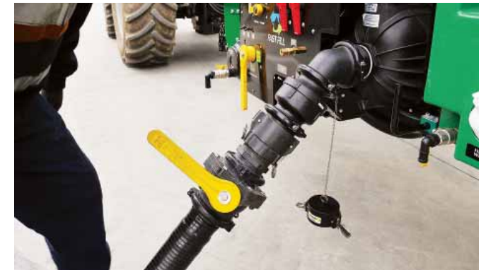
Connect a 3" suction hose to the 'Clean Fill Inlet' and provide at least 500 litres of clean water in the product tank before adding chemicals.
