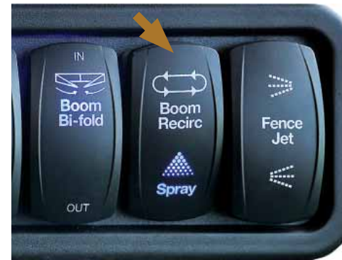
Press the 'Boom Recirc' push button to start boom recirculation.
