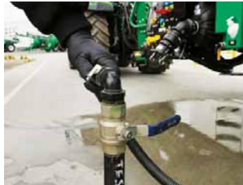
On completion of rinsing, close the Probe valve.
