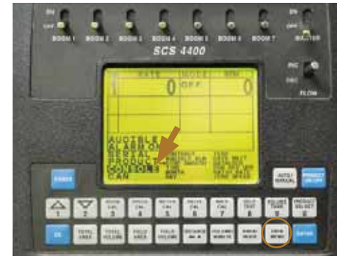
Press the 'DATA MENU' touch button to display the Data Sub Menus - 3rd displayed & highlighted is 'CONSOLE'.
