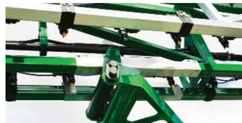
Inner boom folded & supported on the boom rest.
