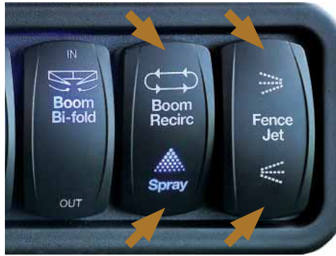
Use the push buttons start Boom Recirculation, then 'Spray' when required.
