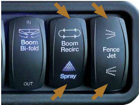
Press the 'Boom Recirc', 'Spray' & 'Spray Jet' push buttons to clean the boom lines & nozzles.
