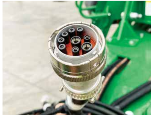
Standard 9 pin ISO BUS connector.
