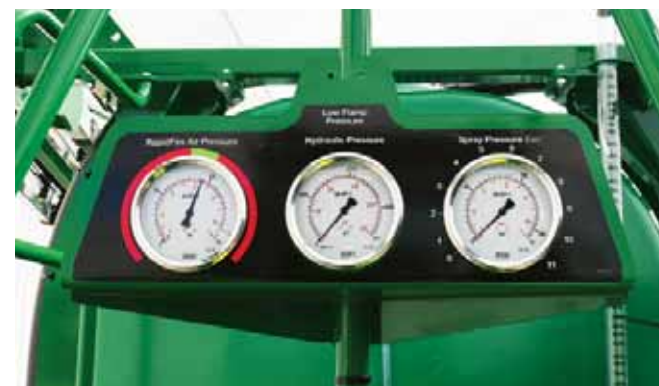
L to R: RapidFire air pressure gauge, Hydraulic pressure gauge (pump) & Spray pressure gauge - located at the front of the Prairie Special for spraying information.
