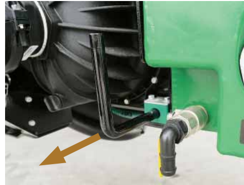
Pull out the 'Main Tank Drain Valve Lever' to safely & completely drain the Product Tank, then close the valve.
