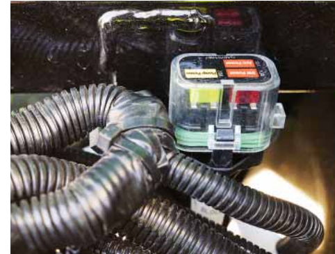
Pump & switch fuse pod located under the Fast Fill Station cover.
