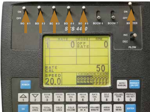
Move the 'BOOM sections' (1-5) & 'Master Switch' toggle switches to On.
