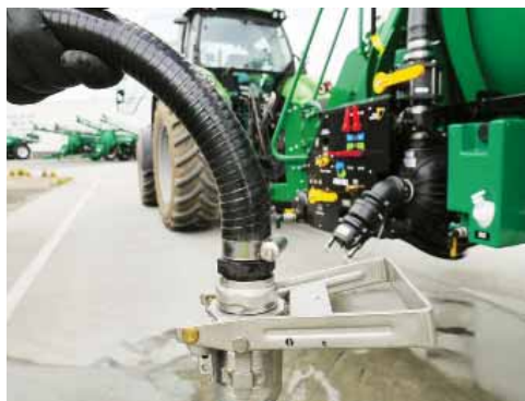
Disconnect the micromatic hose from the chemical source, then rinse the hose.
