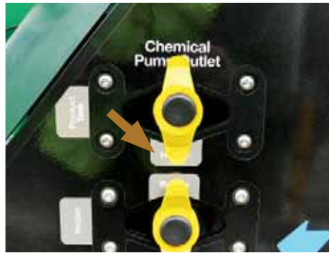
Rotate the 'Chemical Pump Outlet' valve to 'Hopper'.
