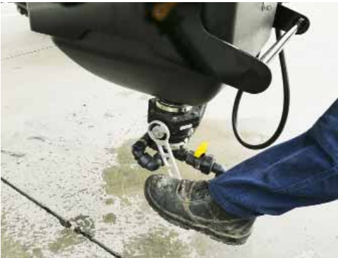
On completion, Close the 'Bottom Drain' valve & 'Bottom Hopper Drain' valve, then refit the camlock cap.
