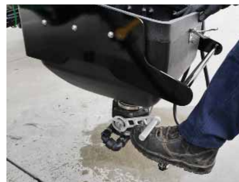
Lift-up to Open the foot operated ball valve at the bottom of the hopper.
