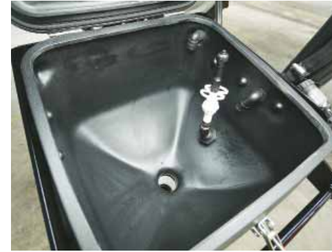
Release the latch & open the Hopper lid.
