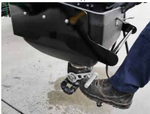
Lift-up to Open the foot operated ball valve at the bottom of the hopper.
