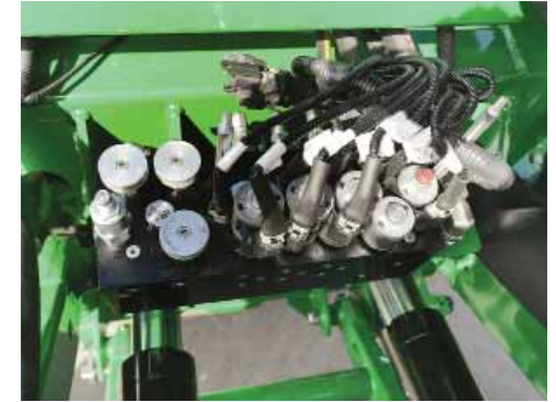
Rear Manifold on top & in the front of the boom centre section.
