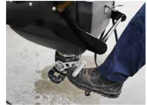
Empty Hopper rinse by transferring its contents to the Product Tank.
